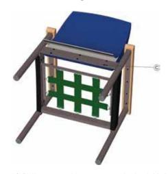
**C:** Using a #2 Philips screwdriver, remove the back(s) (six screws each) from the chair frame.
