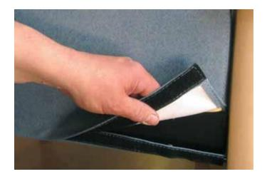
**B:** Separate the Velcro® at the bottom of the seat back cover to reveal the fasteners attaching the seat back to the frame.
