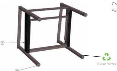
**F & G:** Using a #2 Philips screwdriver, remove the plastic trim panels from the chair frame.
